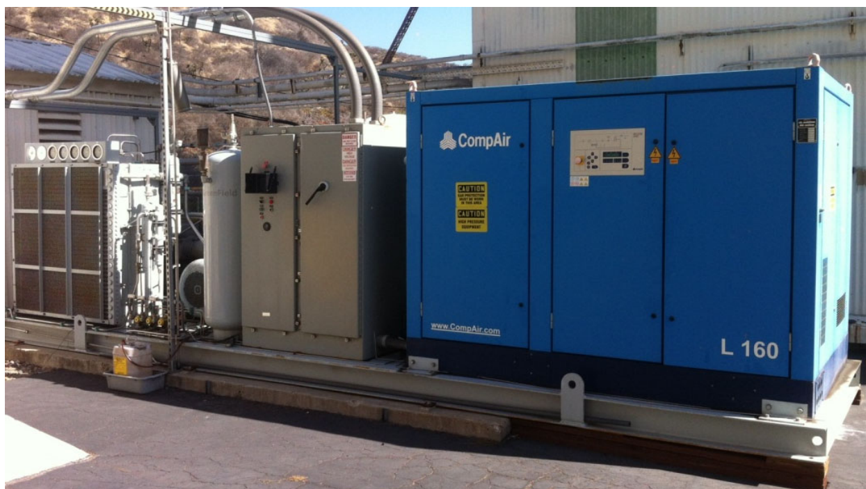
Figure 3. Pilot-Plant iSCWO Compressor Skid
